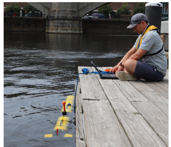
The i3XO EcoMapper gathers up to eight water quality parameters beneath the surface with its nose-mounted EXO1 sonde, and charts of the banks and bed with its bottom mapping system and side-scan sonar.
