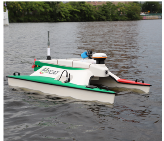
This HYCAT Autonomous Surface Vehicle helps CRWA researchers generate high resolution water quality, bathymetry, and flow data at once along the river.
