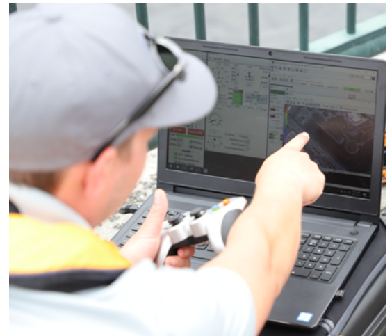
Innovative software allows the technician to plot a course for the autonomous systems using a georeferenced image of the study area.
